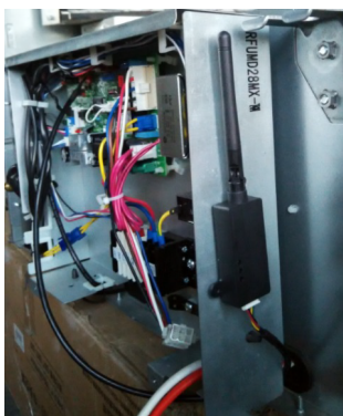
Installation Location Diagram of IDU Wireless Module
